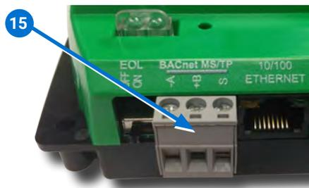
**NOTE:** Use 18 gauge AWG shielded twisted pair cable with maximum capacitance of 51 picofarads per foot (0.3 meters) for all network wiring (Belden cable #82760 or equivalent).
