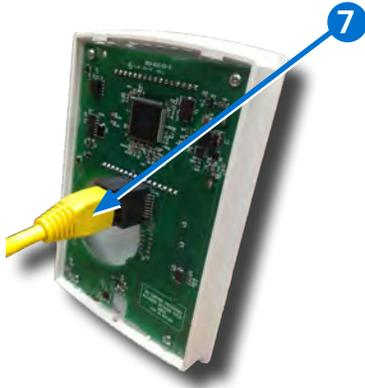
**NOTE:** The Ethernet patch cable should be a maximum of 150 feet (45 meters).
