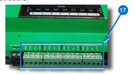
**NOTE:** Wire the HPO-6701 triac and HPO-6703/6705/670 output override boards to the Switched Common SC not the Ground Common **GND** terminal.
