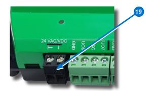
**NOTE:** Connect only one expansion module to each 24 VAC, Class-2 transformer with 12-24 AWG copper wire.
