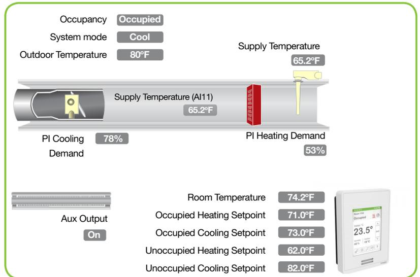
Figure-1 GUI Example - SER8300X
