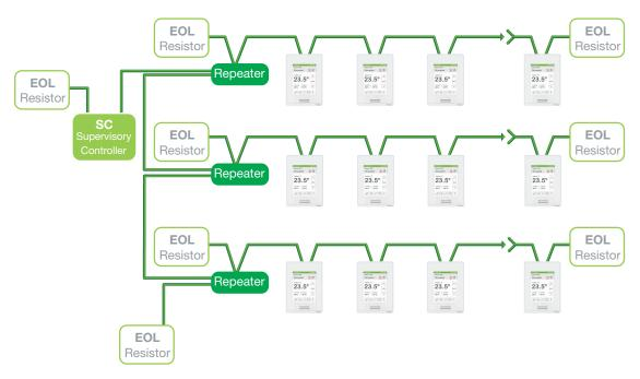
Figure-5 Correct Repeater Use in an EIA-485 Network
