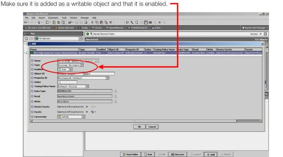
Now when binding your logic block simply point to the relinquish default property of an object at the "fallback" value. This will directly issue the write command to the relinquish default property value insuring you are not locking down the application at priority array 16.
