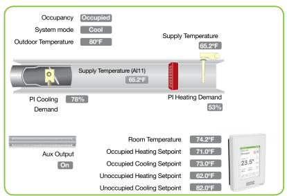
Figure-1 GUI Example - SER8300X
