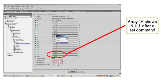
As such, the controller now has an entry in priority array 16 of an object which effectively <u>"overrides"</u> it and <u>by-passes</u> the local control application program.
