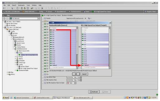
Binding a logic block or function to the "fallback" sets the same behaviour as using the Niagara "set" command. The local server issues a BACnet write command to the controller **without** specifying any
