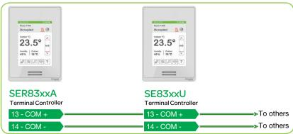
Figure-7 MS/TP Connections
