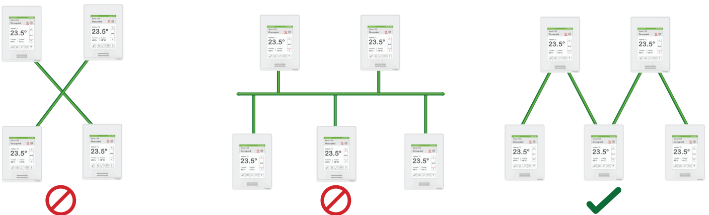
Figure 3 : Three different network configurations: star, bus, and daisy chain. Only the daisy chain configuration is correct for an EIA-485 network
