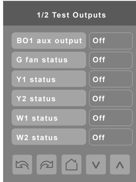
**Note 1:** The test output screen allows manual override of specified outputs. When any BACnet® network priority array includes a value, the status background shows in red. After any output state is overridden, the command is cancelled after 1 minute of screen inactivity (auto exit to main screen) or when page is exited. Refer to the BACnet® integration guide for more details.
