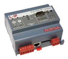
After installation, the L-IP is ready to route packets between the CEA-709 network and the IP network. Thus, all CEA-709 networks connected to L-IPs can exchange data over the CEA-852 channel. If connected to untrusted networks, such as the Internet, all CEA-852 packets can be authenticated by an MD5 checksum and time stamps.
