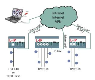
Flat network architectures based on an IP Backbone are specified for best performance and a better maintainability of CEA-709 networks. To meet these requirements, LOYTEC offers a range of IP-Router supporting up to four twisted pair channel.
