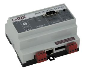
to host customized pages with dynamic content. These pages are accessed by the L-WEB application (.NET). It runs on Windows PCs and Windows Mobile handhelds. The graphical user interface LWEB-800 uses standard Web technologies to visualize and control data in dynamic pages by one or multiple Automation Servers.
