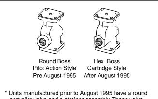
\* Units manufactured prior to August 1995 have a round port pilot valve and a strainer assembly. These valve and strainer assemblies can be replaced with the current hex port cartridge valve and strainer assembly. **Combination Mechanical Water Feeder/** Low Water Cut-Offs
