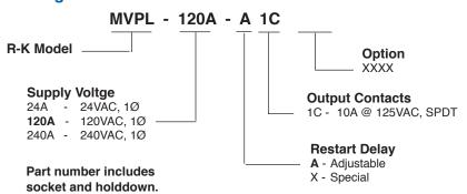
\* For Line Voltages over 300 volts use 600V OT-08 socket.
