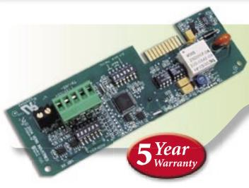
With the optional Communications Board, H8100 Series Energy Meters connect easily to a control/data systems network. It reports energy and power diagnostic information including kW, kWh, kVAR, PF, Amps, Volts, and more.
