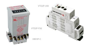
The Veris VTD Series are multi-function time delay relays equipped with an external control switch input and designed for easy socket/DIN mounting. The VTD2P-F50 includes five functions shown at left, while the VTD1P-UNI and VTD2P-UNI include the same five as the VTD2P-F50 plus five more, for the most versatile relay available. Save inventory costs by purchasing one relay for all the functions you need.
