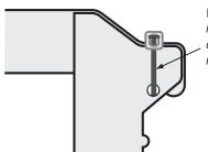
Wire tie used to secure I-Bar in applications where a fault current could exceed 20X rated current.
