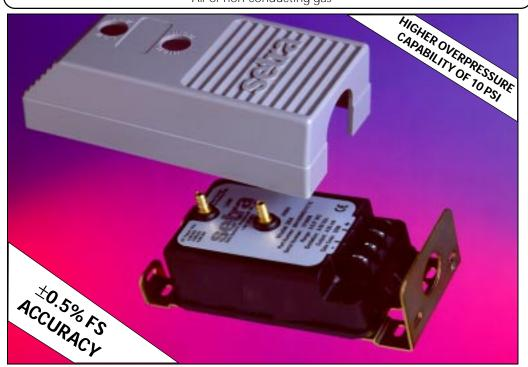
etra Systems 264 pressure transducers sense differential or gauge (static) pressure and convert this pressure difference to a proportional electrical output for either unidirectional or bidirectional pressure ranges. The 264 Series is offered with a high level analog 0 to 5 VDC or 4 to 20 mA output.
