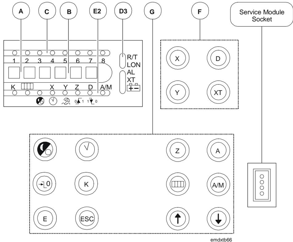
Figure 51: Front Panel Layout
