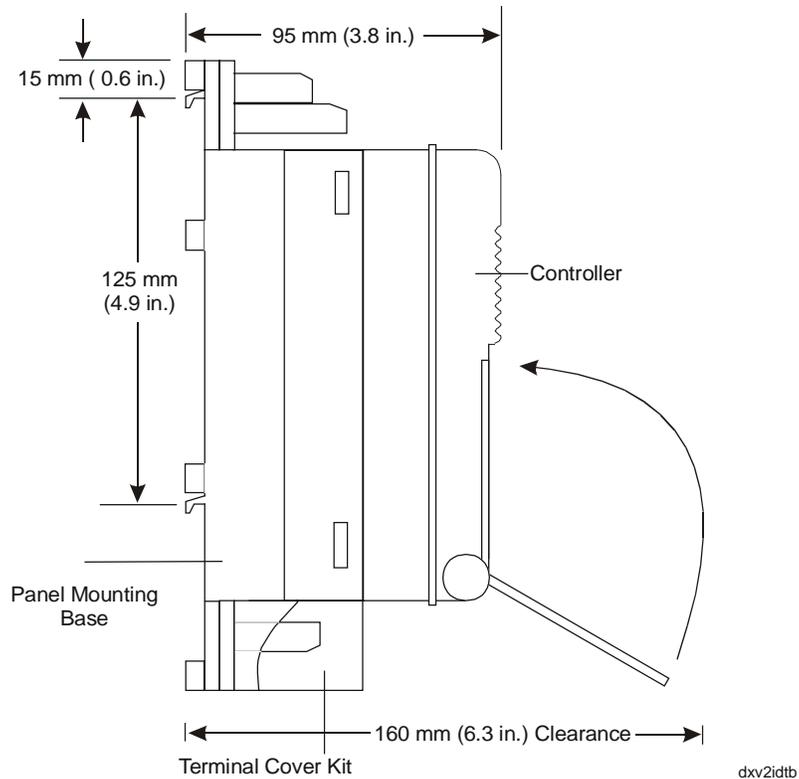
**Figure 2: Installation Details of DX-9200 with Panel Mounting Base**
