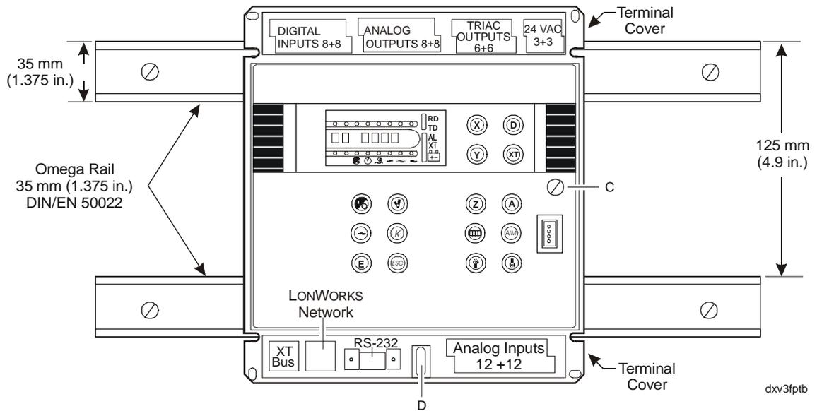
**Figure 3: DX-9200 with Panel Mounting Base on DIN Rails**
