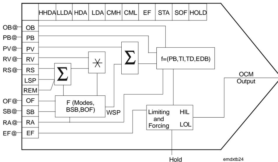
**Figure 18: Control Module Block Diagram**
