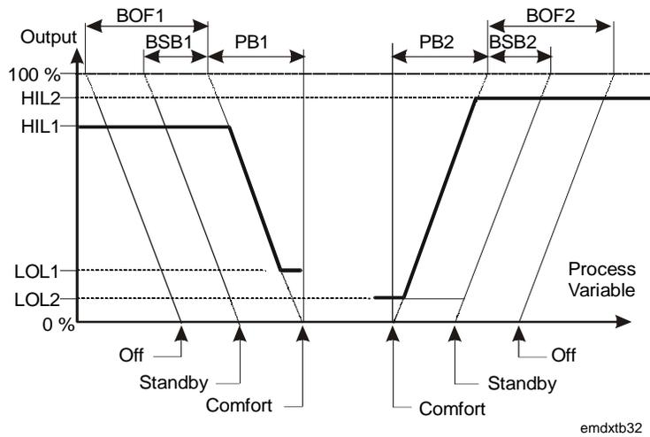
**Figure 24: Heating/Cooling PID Module Operation**
