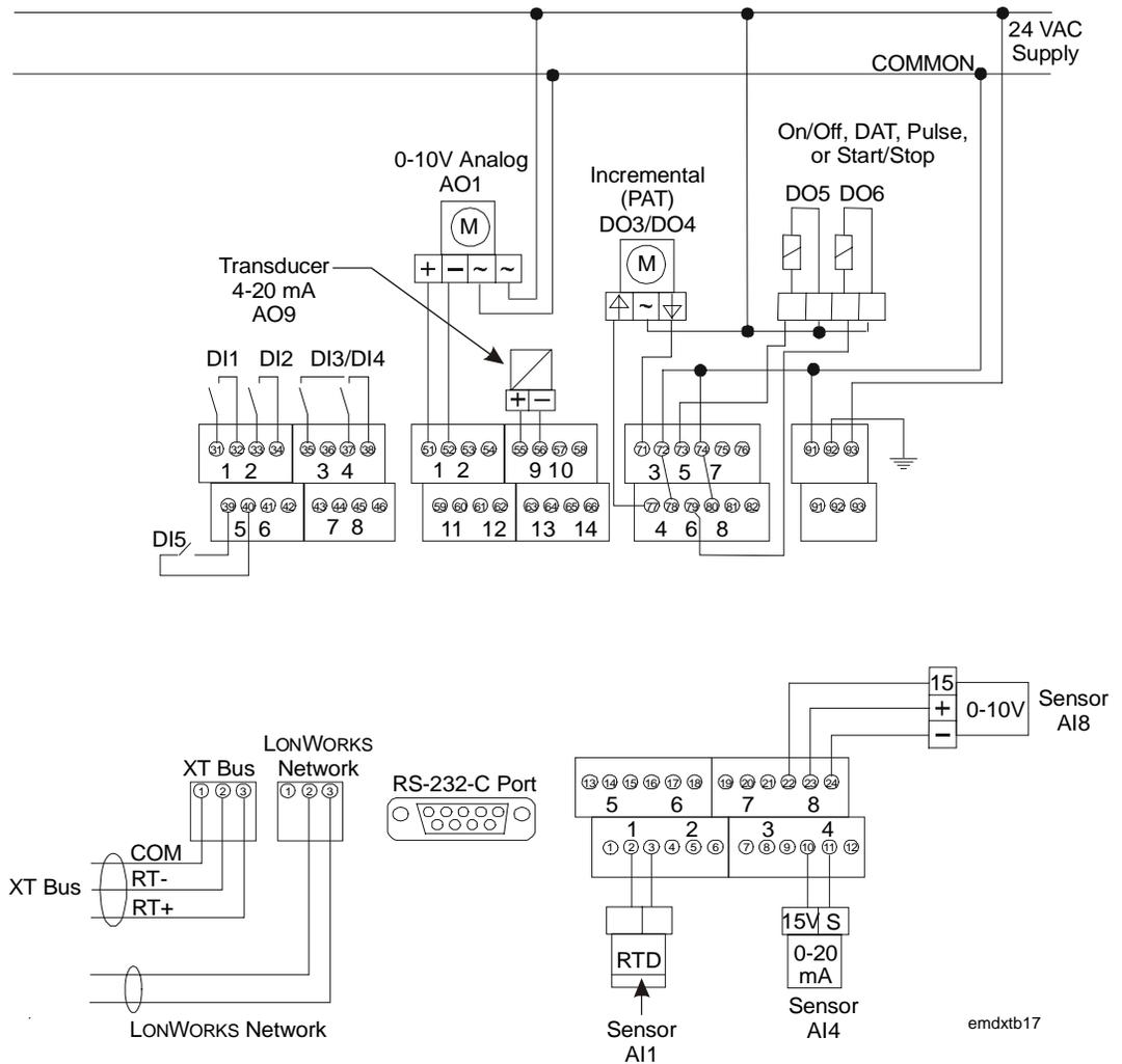
**Figure 11: Wiring Example (Panel Mounting Base Terminals Shown)**
