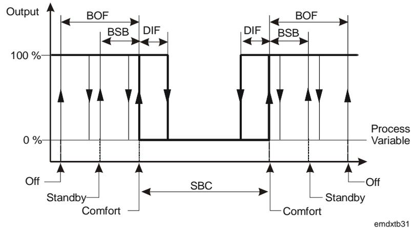
**Figure 23: On/Off Controller with Symmetric Operation (ACT = -1)**
