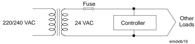
**Figure 13: Incorrect Wiring of Controller to 24 V Transformer**
