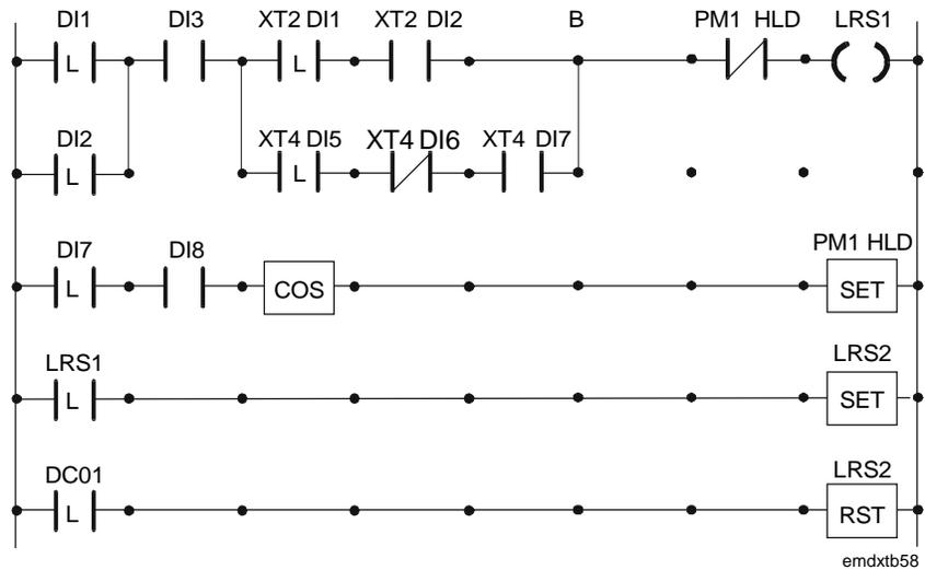
**Figure 50: Example of a PLC Program**
