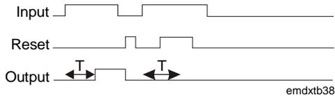
**Figure 30: On Delay with Memory**
