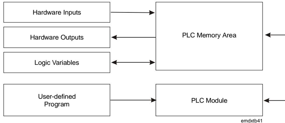
**Figure 33: Programmable Logic Control**
