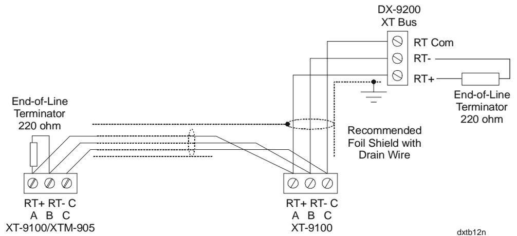
**Figure 7: Connection Details for the XT Bus**
