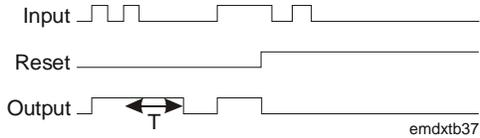
**Figure 29: Retriggerable Pulse**
