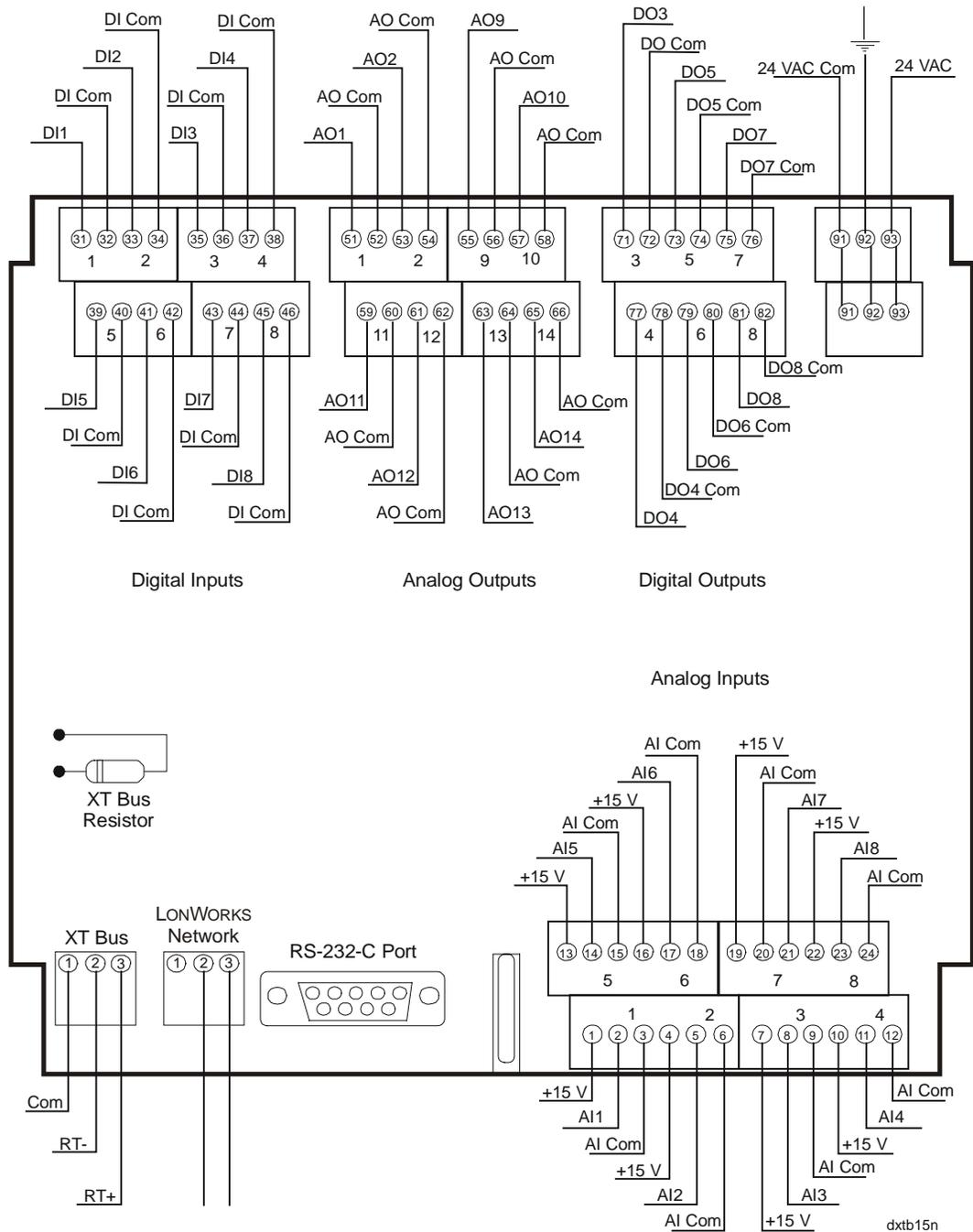
**Figure 5: Connections at the Top and Bottom of the Panel Mounting Base**
