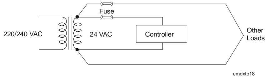
**Figure 12: Correct Wiring of Controller to 24 V Transformer**
