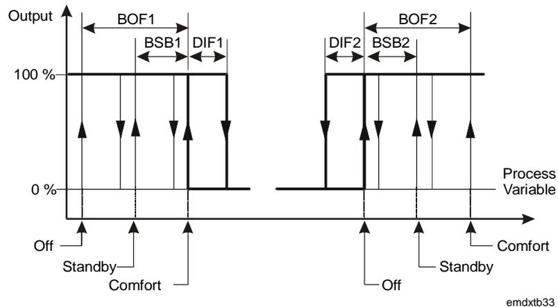
**Figure 25: Heating/Cooling On/Off Module Operation**
