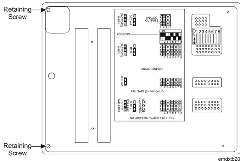
**Figure 14: Retaining Screws on the Back of the Controller**
