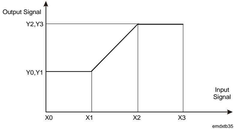
**Figure 27: Example of a Line Segment Function**
