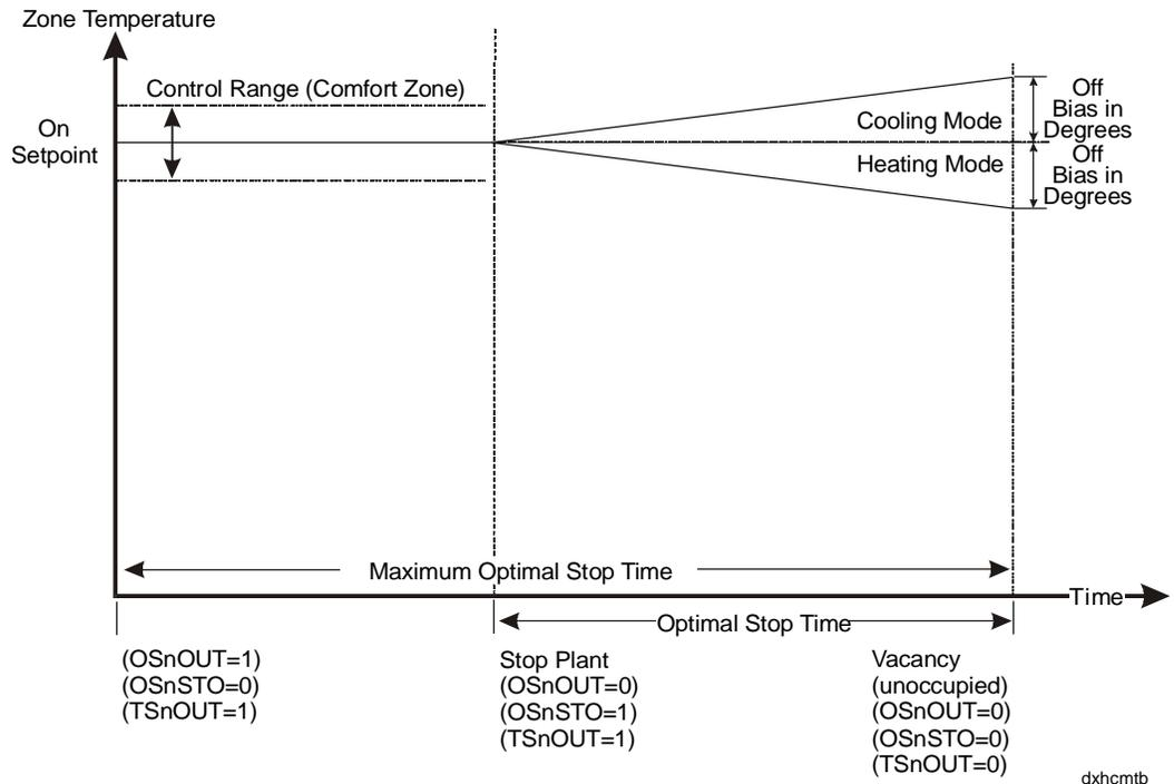
**Figure 17: Optimal Stop Module in Heating/Cooling Mode**
