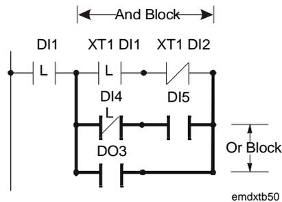
Figure 42: OR Block Nested Within AND Block
