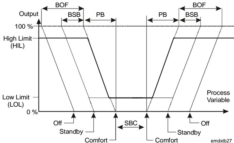
**Figure 20: Controller with Symmetrical Operation (Proportional Controller Only)**
