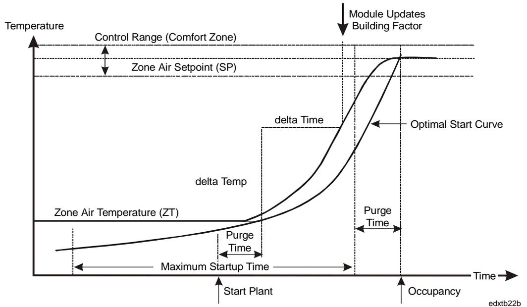
**Figure 16: Optimal Start Module in Heating mode**
