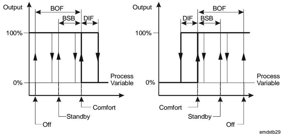
**Figure 22: Reverse Acting Controller/Direct Acting Controller**
