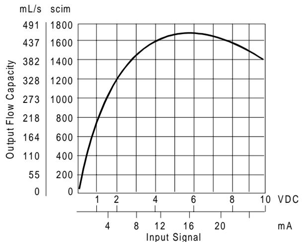
**Figure 5: High-volume Models: Input Signal (volts DC and mA) vs. Output Flow Capacity (scim and mL/s)**
