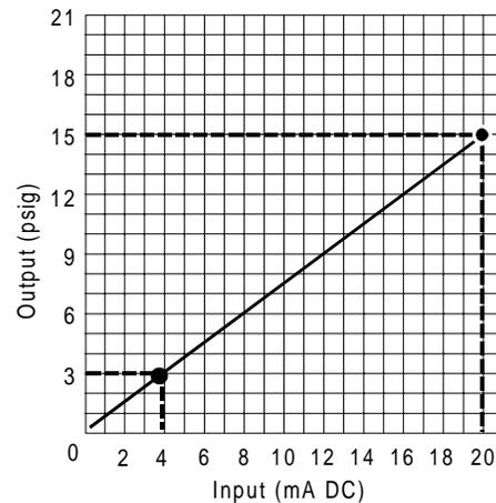
**Figure 4: EP-8000-3 and -4: Input (mA DC) vs. Output (psig)**
