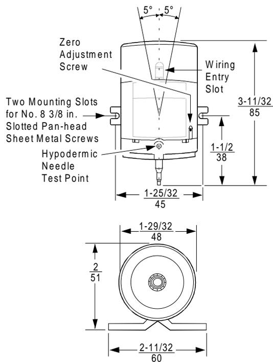
**Figure 6: EP-8000 Low-volume Output Model Dimensions (in./mm)**
