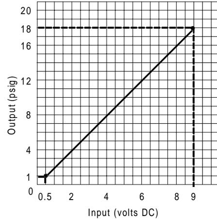
**Figure 3: EP-8000-1 and -2: Input (volts DC) vs. Output (psig)**
