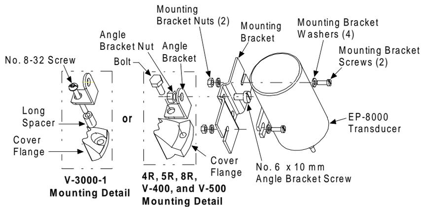
**Figure 8: EP-8000-101 Mounting Kit for Installation of the EP-8000 to a 4R, 5R, 8R, V-400, V-500, or V-3000-1 Valve Actuator with or without a V-9502 Positioner**
