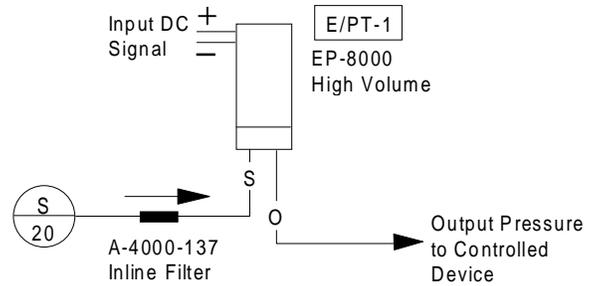
Figure 11: High-volume Models Wiring/Tubing
