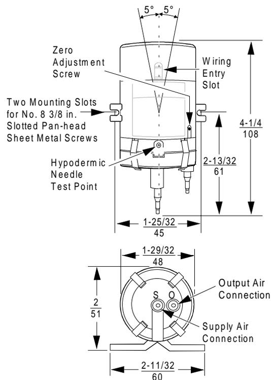
**Figure 7: EP-8000 High-volume Output Model Dimensions (in./mm)**
