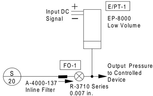
Figure 10: Low-volume Models Wiring/Tubing
