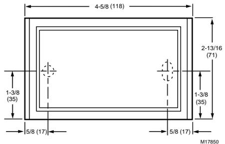
Fig. 1. C7130A,B Wall-Mount Temperature Sensor dimensions in in. [mm].
