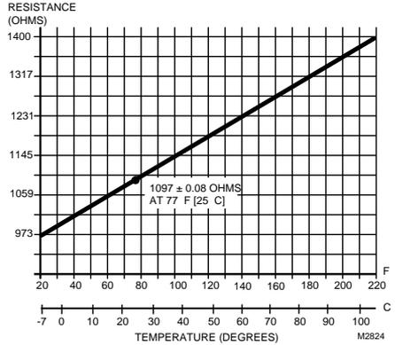
Fig. 5. C7130B resistance vs. temperature performance characteristics.
