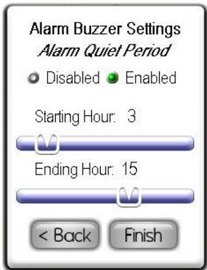
Fig. 20 Specifying Alarm Quiet Period within the Alarm Buzzer Settings
