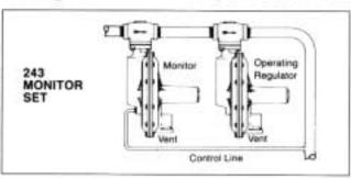
Periodic Inspection: Regulators are pressure control devices with numerous moving parts subject to wear that is dependent upon particular operating conditions. To assure continuous satisfactory operation, a periodic inspection schedule must be adhered to with the frequency of inspection determined by the severity of service and applicable laws and regulations. See Bulletin RM-1306 field service instructions.
